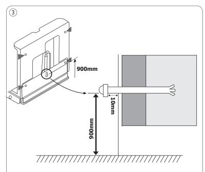
Insert a screw into the lower middle hole, leaving 10mm protruding from the wall surface. Hang the changing station on the screw.
