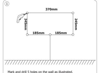
Note: Ensure there is no electric/water pipe beneath the holes.
