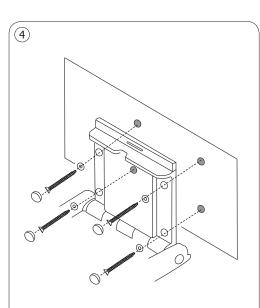
Mount the changing station onto the wall using the 4 side screws and washers.
